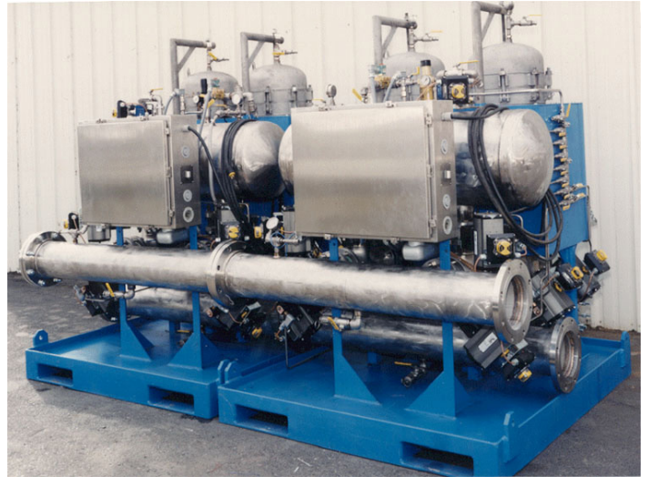
Backwash filtration system
